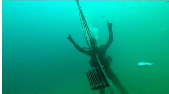
ARMS unit in final stage of original mounting system suspended in water column by 5 gal bucket filled with air
